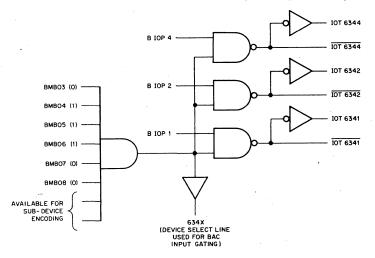
Figure 26. Typical Device Selector (Device 34)
