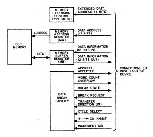
Figure 34. Data Break Transfer Interface Block Diagram
