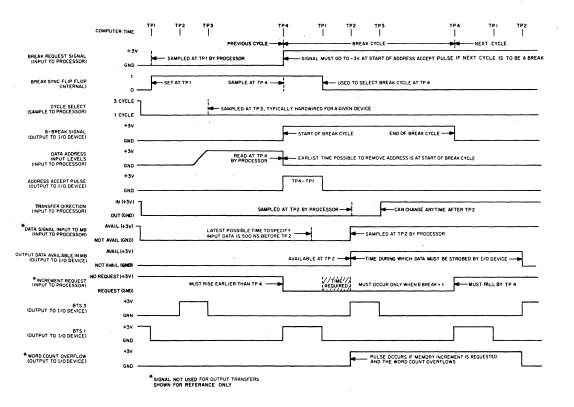
Figure 37. Single-Cycle Data Break Output Transfer Timing Diagram
