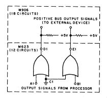
Fig. 45 Typical M623/M906 Positive Output Circuit
