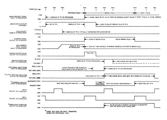
Figure 35. Single-Cycle Data Break Input Transfer Timing Diagram
