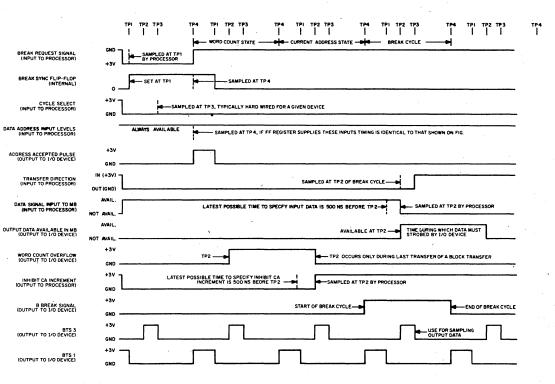
Figure 42. Three-Cycle Data Break Timing Diagram
