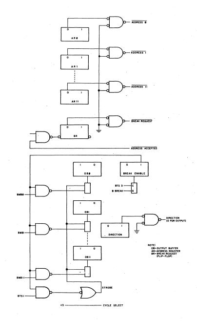
Figure 38. Device Interface Logic for Single-Cycle Data Break Output Transfer
