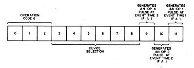
Figure 7. IOT Instruction Bit Assignments
