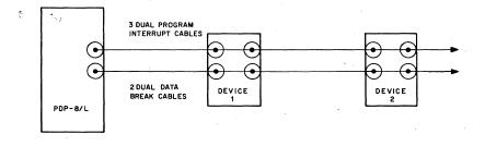
Fig. 49 I/O Bus Configuration
