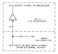
Fig. 43 Typical M111/M906 Positive Input Circuit
